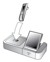
Figure 8: Inserting the headset into the cradle for storage and charging
